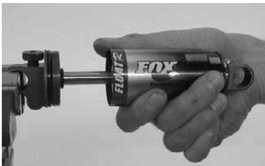
Figure C. Air Sleeve Installation.
