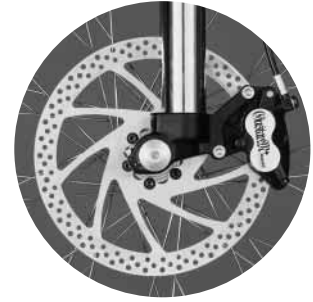
Brake caliper and rotor MAGURA Gustav M
