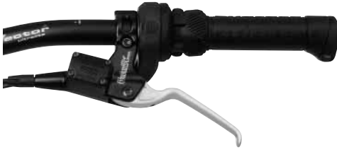
Brake lever (master cylinder) MAGURA Gustav M
