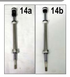
17. Add 3 cc/ml of 15wt oil or RockShox RedRum to the positive air chamber (fig. 17). This lubricates the positive air seal o-ring and protects against heat friction and wear. Install the air top cap with a 24mm socket to 50 in-lbs.
