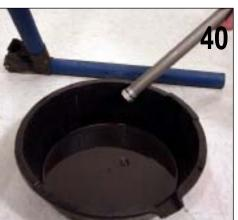
41. Pull the top cap/compression damper assembly slowly out of the Pure tube. You need to pull fairly hard and twist the assembly to work it free from the Pure tube (fig. 41).
