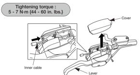
Connect the inner cable to the derailleur as shown in the illustration.
