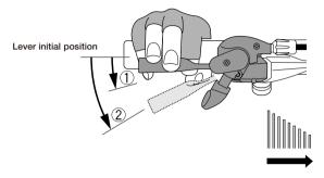
To shift from a small sprocket to a larger sprocket Press lever once to shift one step from a smaller to a larger sprocket.
