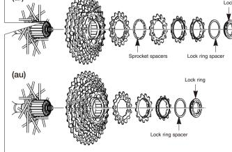
For installation of the sprockets, use the special tool (TL-LR10) to tighten the lock ring.
