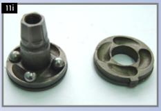
**111:** Before reassembling the rotor unit, smear a small quantity of grease in the seats of the ball bearings.
