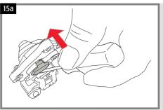
Reassemble the pincer unit onto the fork or the frame respecting the instructions in the braking system manual. Furthermore, effectuate the adjustments mentioned in chapter 5.
