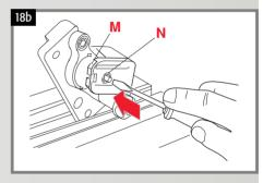
Maintain the pincer unit mounted on a vice with protective pieces as shown in the figure, without tightening too
