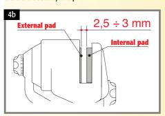
**4b:** Also check that the distance between the pads is always 2.5-3mm as shown in the figure. If the measurement is less, exert a light pressure on the external pad until the pad comes to its resting position. Assemble the front and/or the rear wheel as indicated by the manufacturer.
