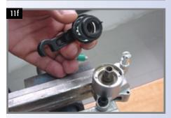
11g: Utilising the tool shown in the figure, unscrew the internal ring (12) in an anti-clockwise direction and remove it.
