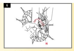
If the action of the lever is too long, repeat the adjustment operations so that the desired situation is obtained.
