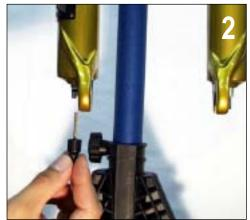
3. Using a 5 mm hex wrench, loosen the right damper shaft bolt five turns or halfway. Using a 10 mm socket, loosen the left shaft nut until it is flush or just beyond with the dual air shaft end.
