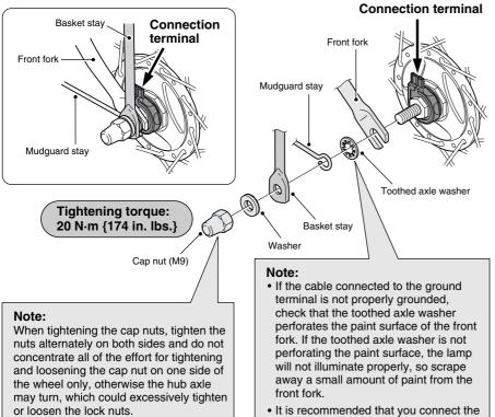
• It is recommended that you connect the two wires to ensure that the current flows smoothly.
