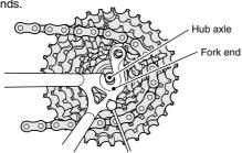
2. Place the non-turn washers onto the right side and left side of the hub axle. At this time, turn the hub axle to install so that the projecting parts of the non-turn washers fit into the grooves of the fork ends.
