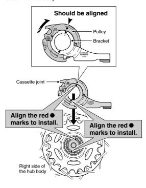
Secure the cassette joint to the hub with the cassette joint fixing ring. When installing the cassette joint fixing ring, align the yellow ● mark with the yellow ● mark on the cassette joint pulley.
