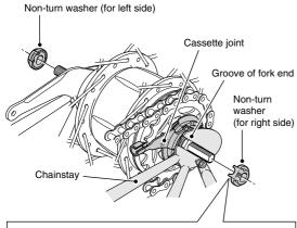
Different types of left and right non-turn washers are available for use with standard and reversed fork ends. Use whichever non-turn washers are suitable.
