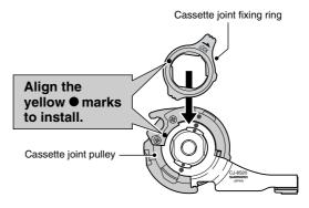
After installing the cassette joint fixing ring, turn it 45° clockwise.
