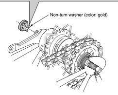
**3.** Screw the flange nuts onto both ends of the hub axle. After this, take up the slack in the chain and then tighten the flange nuts to secure the wheel to the frame.
