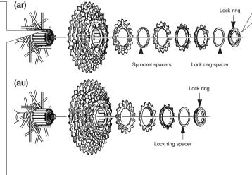
· For installation of the sprockets, use the special tool (TL-LR10) to tighten the lock ring.
