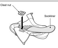
**3.** From the bottom of the shoe, position a cleat and then a cleat adapter over the cleat holes. The cleats are compatible with both left and right pedals. Provisionally tighten the cleat mounting bolts.
