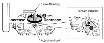
When the bolt is turned clockwise, the spring tension increases and the red part of the tension indicator becomes larger. When the bolt is turned all the way clockwise, it will suddenly become hard to turn. Do not turn the bolt beyond this point. When the bolt is turned counterclockwise, the spring tension decreases and the red part of the tension indicator becomes smaller. Once the red part of the tension indicator can no longer be seen, do not turn the bolt counterclockwise any further.
