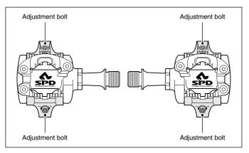
When the adjustment bolt is turned clockwise, the spring tension increases, and when it is turned counterclockwise, the spring tension decreases.
