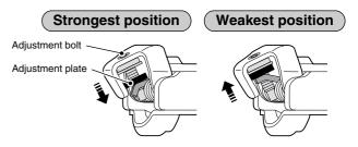
If the adjustment plate is at the strongest or the weakest position, do not turn the adjustment bolt any further.
