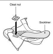
**3.** From the bottom of the shoe, position a cleat and then a cleat adapter over the cleat holes. The cleats are compatible with both left and right pedals. Provisionally tighten the cleat mounting bolts.
