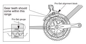
The level section of the chain guide outer plate should be directly above and parallel to the largest chainring. Secure using a 5mm Allen key.
