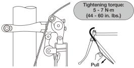
After taking up the initial slack in the cable, re-secure to the front derailleur as shown in the illustration.
