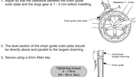
3. Secure using a 5mm Allen key.
