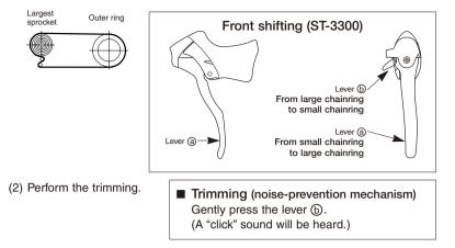
(3) After trimming, adjust the clearance (by using the cable-adjustment bolt) of the chain and chain guide to the minimum (0 - 0.5 mm).
