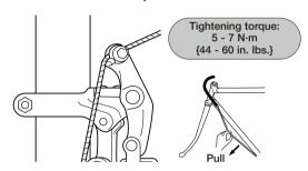
After taking up the initial slack in the cable, re-secure to the front derailleur as shown in the illustration.
