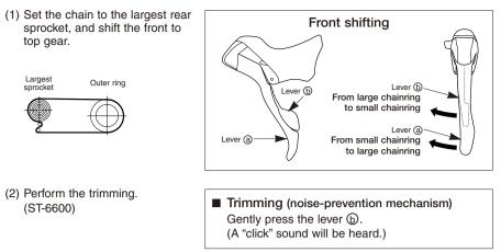
While turning the crank arm, gently operate lever (b) and check that the front derailleur moves slightly toward the small chainring. If the front derailleur moves by a large amount and the chain is set onto the small chainring at this time, loosen the top adjustment bolt by 1/8th of a turn. Then, after returning the chain to its original position, adjust and check the trimming mechanism.
