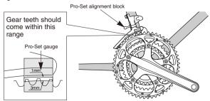
The level section of the chain guide outer plate should be directly above and parallel to the largest chainring. Secure using a 5mm Allen key.
