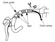
6. Finally, wrap the handlebar with the finish tape.
