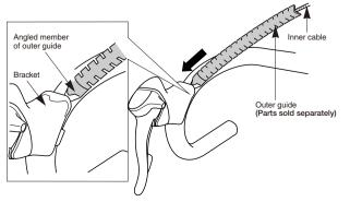
4. Set the outer casing on the inner cable, and in the bracket along the outer guide.
