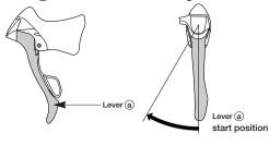
If operation of lever (a) dose not complete the chainring shift stroke, operate lever (a) again for the distance (X') to complete that part of the lever stroke (X) which was short.
