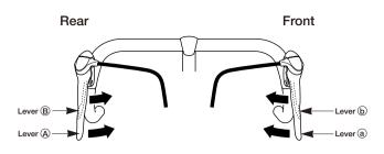
Lever (A): Shifts from smaller to larger rear sprocket. Lever (B): Shifts from larger to smaller rear sprocket. Lever (a): Shifts from smaller to larger chainring. Lever (b): Shifts from larger to smaller chainring.
