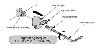
Install with the adjustment bolt tightened. The adjustment range for the adjustment bolt is six full turns.
