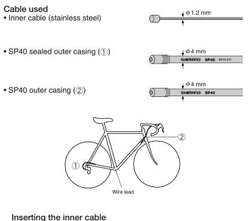
Insert the inner cable into the outer casing from the end with the marking on it. Apply grease from the end with the marking in order to maintain cable operating efficiency.
