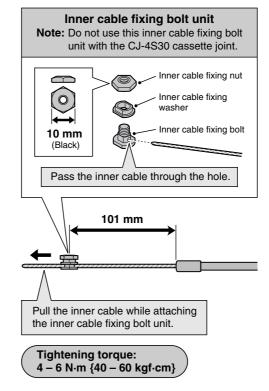
7. Bring the cable around to the cassette joint pulley, hold so that the inner cable fixing nut is facing to the outside (toward the fork end), and then slide the flats part of the inner cable fixing washer into the gap in the pulley.
