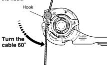
**9.** Attach the inner cable to the pulley as shown in the illustration, pass the inner cable through the slit in the cassette joint bracket, and then insert the end of the outer casing securely into the outer casing holder.
