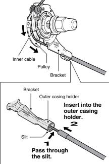
If first inserting the outer casing into the outer casing holder is easier, then first insert the outer casing into the outer casing holder, and then insert a 2 mm Allen key or a #14 spoke into the hole in the cassette joint pulley, and then turn the pulley so that the inner cable fixing bolt unit fits into the gap in the pulley.
