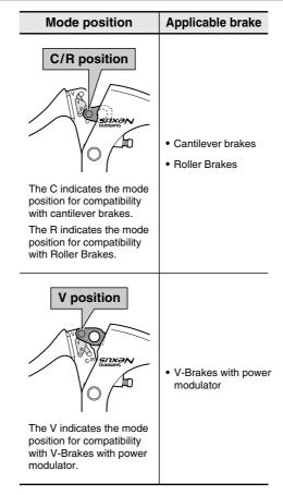
Use the brake levers with mode switching mechanism in the combinations given above.
