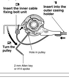
Note: Check that the inner cable is correctly seated inside the pulley guide.
