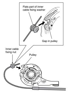
8. Turn the cable 60° counterclockwise and attach it to the hook.
