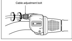
2. After adjusting the cassette joint, cut off the excess length of inner cable and then install the inner end cap.
