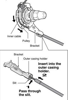
If first inserting the outer casing into the outer casing holder is easier, then first insert the outer casing into the outer casing holder, and then insert a 2 mm Allen key or a #14 spoke into the hole in the cassette joint pulley, and then turn the pulley so that the inner cable fixing bolt unit fits into the gap in the pulley. З Insert into the Insert the inner cable outer casing fixing bolt unit holder 00000 2 Turn the
