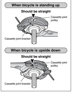
If the yellow setting lines are not aligned, turn the cable adjustment bolt of the Revoshift lever to align the setting lines. After this, move the Revo-shift lever once more from [4] to [1] and then back to [4], and then recheck to be sure that the yellow setting lines are aligned.
