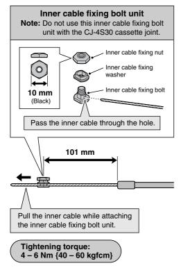
7. Bring the cable around to the cassette joint pulley, hold so that the inner cable fixing nut is facing to the outside (toward the fork end), and then slide the flats part of the inner cable fixing washer into the gap in the pulley.
