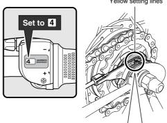
The yellow setting lines on the cassette joint are located in two places. Use the one that is easiest to see.
