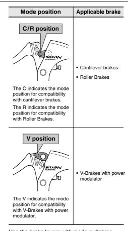
Use the brake levers with mode switching mechanism in the combinations given above.
