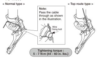
After taking up the initial slack in the cable, re-secure to the front derailleur as shown in the illustration.
