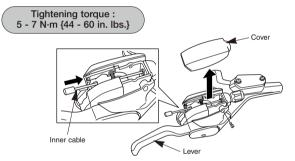
Connect the inner cable to the derailleur as shown in the illustration.
