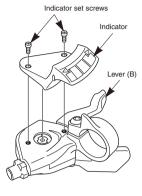
Check the operation of the indicator. If it does not operate correctly, re-install the indicator while taking particular note of steps 3. to 4.
