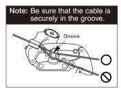
Connect the cable to the rear derailleur and, after taking up the initial slack in the cable, re-secure to the rear derailleur as shown in the illustration.
