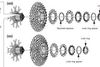
For installation of the sprockets, use the special tool (TL-LR15) to tighten the lock ring.
