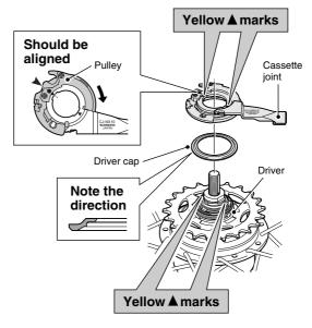
1) Secure the cassette joint to the hub with the cassette joint fixing ring. When installing the cassette joint fixing ring, align the yellow ● mark with the yellow ● mark on the cassette joint pulley.
