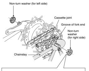
Different types of left and right non-turn washers are available for use with standard and reversed fork ends. Use whichever non-turn washers are suitable.
