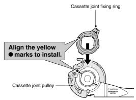
After installing the cassette joint fixing ring, turn it 45° clockwise.
