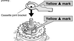
Secure the cassette joint to the hub with the cassette joint fixing ring. When installing the cassette joint fixing ring, align the yellow ● mark with the yellow ● mark on the cassette joint bracket. After installing the cassette joint fixing ring, turn it 45° clockwise.
