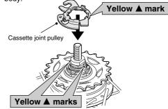
2. Align the yellow ▲ mark on the cassette joint bracket with the yellow ▲ mark on the cassette joint pulley.
