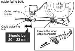
6. Check that both ends of the outer casing are securely inserted into the cable adjusting bolts of both the brake lever and brake arm.
