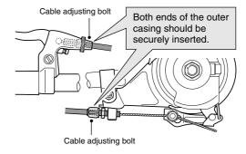
7. Push the link back until it stops. Then, while pulling the inner cable to apply the full amount of tension to the cable, tighten the inner cable fixing nut.
