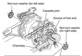
• Different types of left and right non-turn washers are available for use with standard and reversed fork ends. Use whichever non-turn washers are suitable.
