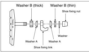
**3.** While holding the shoe against the rim, tighten the shoe fixing nut.
