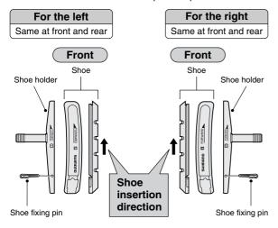
**3.** Insertion of shoe fixing pin is very critical to keep shoe properly fixed in place.
