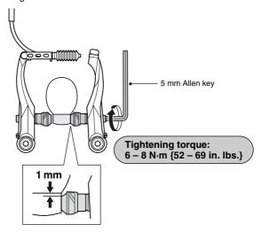
Pass the inner cable through the inner cable lead, and after setting so that the total of the clearances between the left and right shoes and the rim is 2 mm, tighten the cable fixing holt
