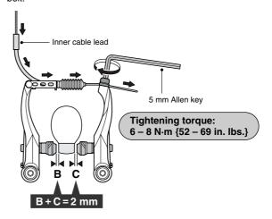
**5.** Adjust the balance with the spring tension adjustment
