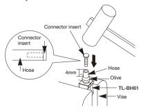
5. After checking that the olive is positioned as shown in the illustration, apply grease to the threads of the connecting bolts and then attach the hoses to the brake lever and calipers as shown in the illustration.
