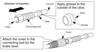
3. In order to check that the ends of the hose are fitted securely into the base of the hose mounts of the calipers and brake lever, make marks on the hose beforehand as shown in the illustration. (As a guide, the length of hose inside the mounts should be approximately 14 mm, measured from the cut end of the hose.)
