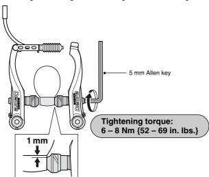
**4.** Pass the inner cable through the inner cable lead, and after setting so that the total of the clearances between the left and right shoes and the rim is 2 mm, tighten the cable fixing bolt.
