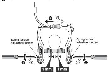
**6.** Depress the brake lever about 10 times as far as the grip and check that everything is operating correctly and that the shoe clearance is correct before using the brakes.
