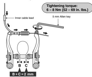
5. Adjust the balance with the spring tension adjustment screws.
