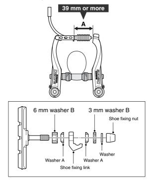
3. While holding the shoe against the rim, tighten the shoe fixing nut.
