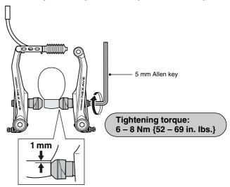
**4.** Pass the inner cable through the inner cable lead, and after setting so that the total of the clearances between the left and right shoes and the rim is 2 mm, tighten the cable fixing bolt.
