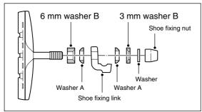
3 While holding the shoe against the rim, tighten the shoe fixing nut.
