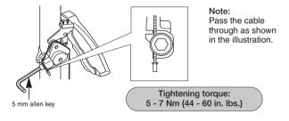
After taking up the initial slack in the cable, re-secure to the front derailleur as shown in the illustration.
