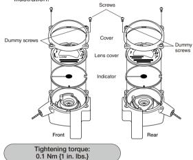
Turn the pulley and remove the cable as shown in the illustration. Turn the pulley clockwise, and then insert the end of the new cable until it is in the position shown in the illustration. Install the indicator, lens cover and cover in that order.
