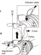
5. Making fine adjustments to the indicator cable The indicator cable is equipped with an adjustment bolt. Turn the adjustment bolt to adjust to the optimum setting so that the needle points to "2" (at both front and rear).
