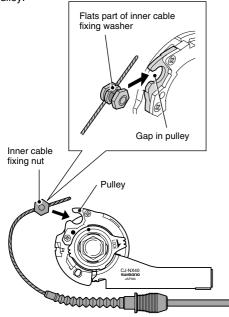
7. Turn the cable 60° counterclockwise and attach it to the hook.
