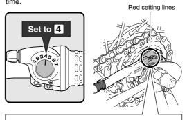
The red setting lines on the cassette joint are located in two places. Use the one that is easiest to see.
