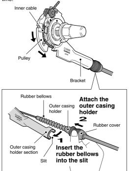
If first inserting the outer casing holder into the outer casing holder section of the cassette joint is easier, then first insert the outer casing holder into the outer casing holder section of the cassette joint, and then insert a 2 mm Allen key or a #14 spoke into the hole in the cassette joint pulley, and then turn the pulley so that the inner cable fixing bolt unit fits into the gap in the pulley.
