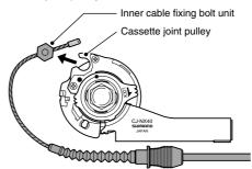
If it is difficult to pull the outer casing holder out from the outer casing holder section of the cassette joint, insert a 2 mm Allen key or a #14 spoke into the hole in the cassette joint pulley, and then turn the pulley to loosen the inner cable. Then remove the inner cable fixing bolt unit from the pulley first, and after this remove the outer casing holder from the outer casing holder section.
