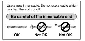
While holding the end of the rubber bellows, insert the inner cable. Be careful not to pierce the rubber bellows with the end of the inner cable at this time.
