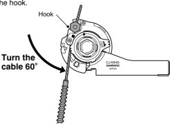
**8.** Attach the inner cable to the pulley as shown in the illustration, pass the part of the inner cable which has the rubber bellows attached through the slit in the cassette joint bracket, and then insert the outer casing holder securely into the outer casing holder section. Be careful not to damage the rubber bellows at this time
