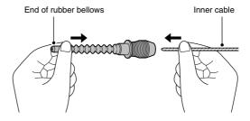
2) Slide the rubber bellows onto the inner cable.
