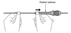
3) Push the outer casing on so that it securely touches the outer casing holder.
