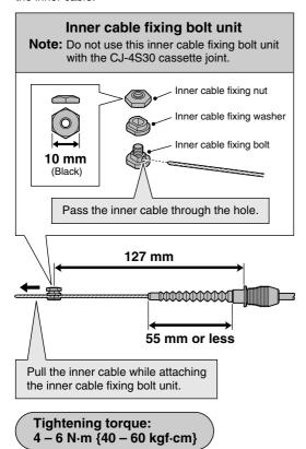
6. Bring the cable around to the cassette joint pulley, hold so that the inner cable fixing nut is facing to the outside (toward the fork end), and then slide the flats part of the inner cable fixing washer into the gap in the pulley.
